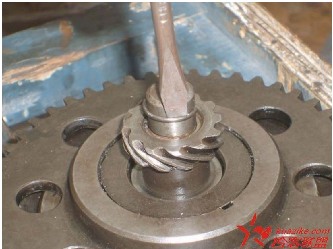
装入钢丝卡环 Pushing the circlip in place.
