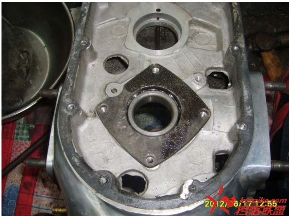
装上曲轴前轴承压板。 Put the bearing retaining plate in place.
