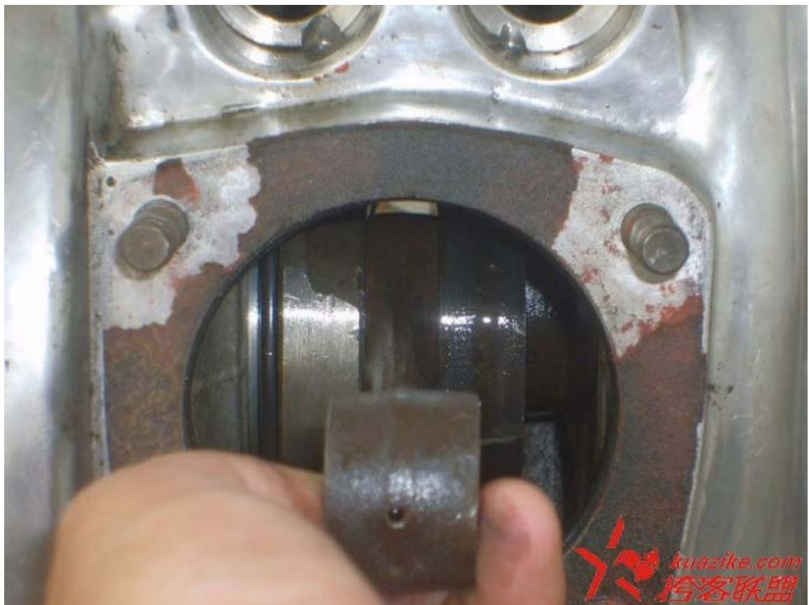
检查连杆大头的径向间隙 Check the connecting rods for in-and-out free play.
