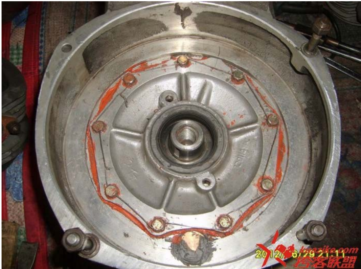
Bolt on the bearing cover plate.
