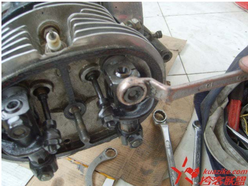
用15的扳手拆下摇臂固定螺母暨缸盖固定螺母 Use a 15mm wrench to remove the rocker arm / cylinder head nuts.
