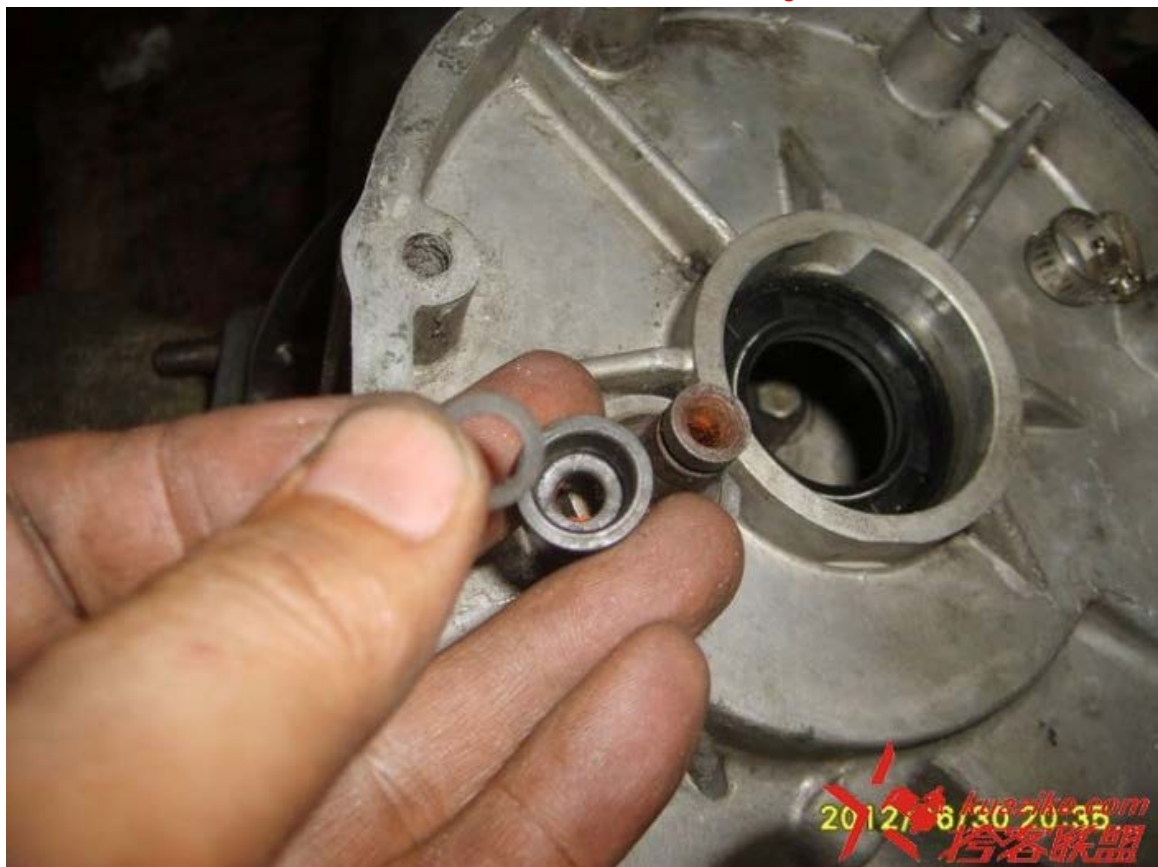
经过检查，这个橡胶油道接口有点短，高度不足，手头没有配件，临时内部加了一个一毫米粗的密封圈垫高。 An inspection showed that the oil seal was a bit too short, so a 1mm thick washer was added.
