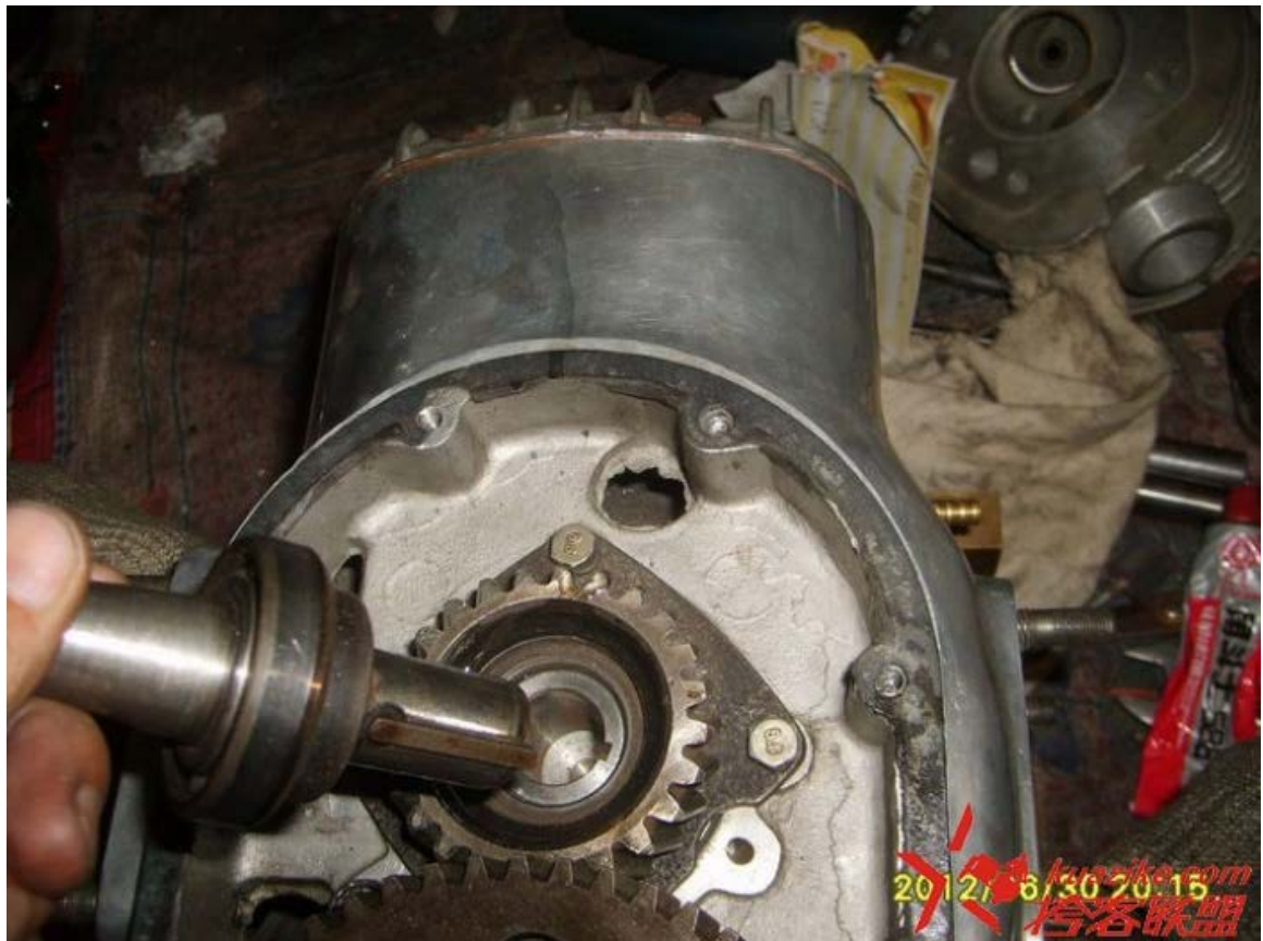
装上发电机轴，注意先装好定位键。 Insert the alternator shaft, paying attention to properly align the Woodruff key.
