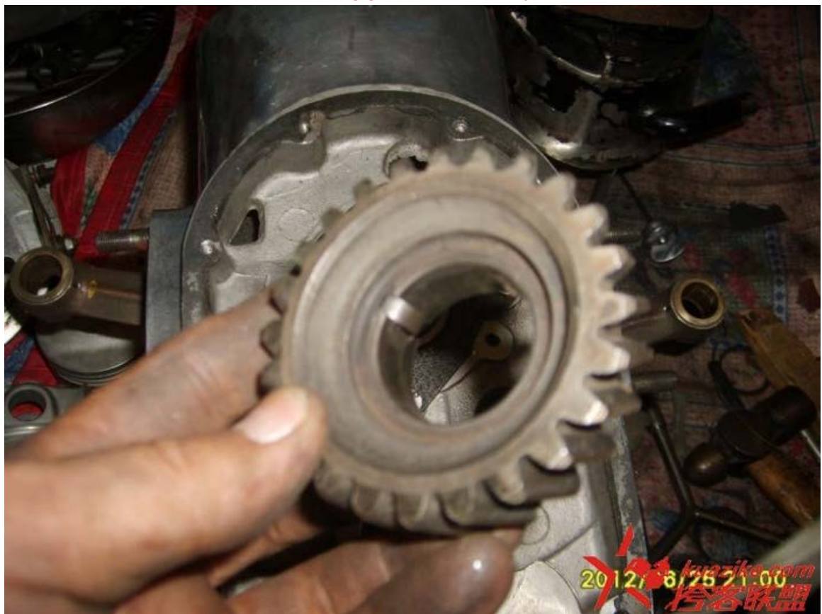
装上曲轴 正时齿轮的定位键。 Place the timing gear's Woodruff key on the shaft.
