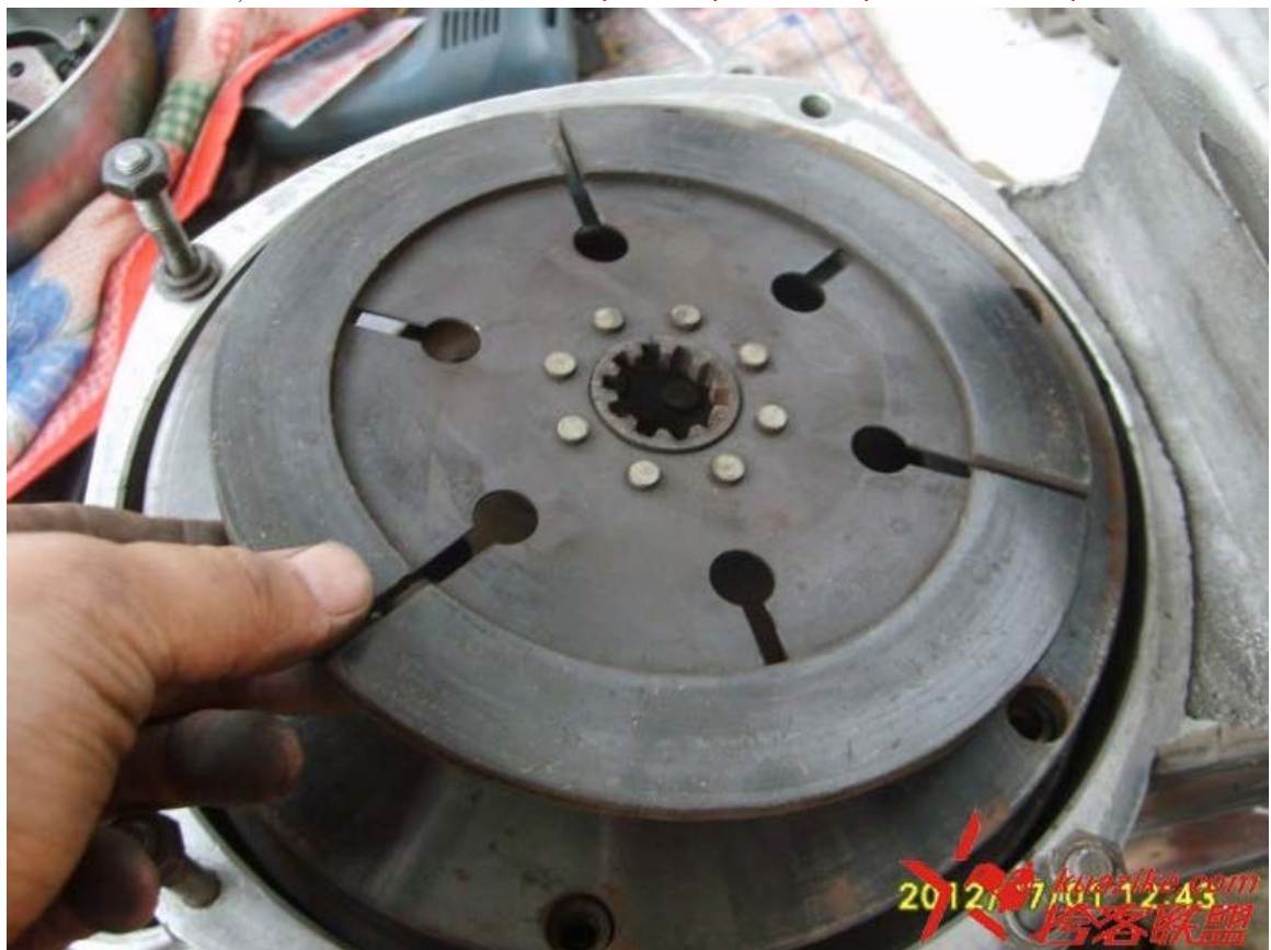
放上第二片离合片，也是突出一面朝向飞轮。The friction plates go on with the rivet side out.
