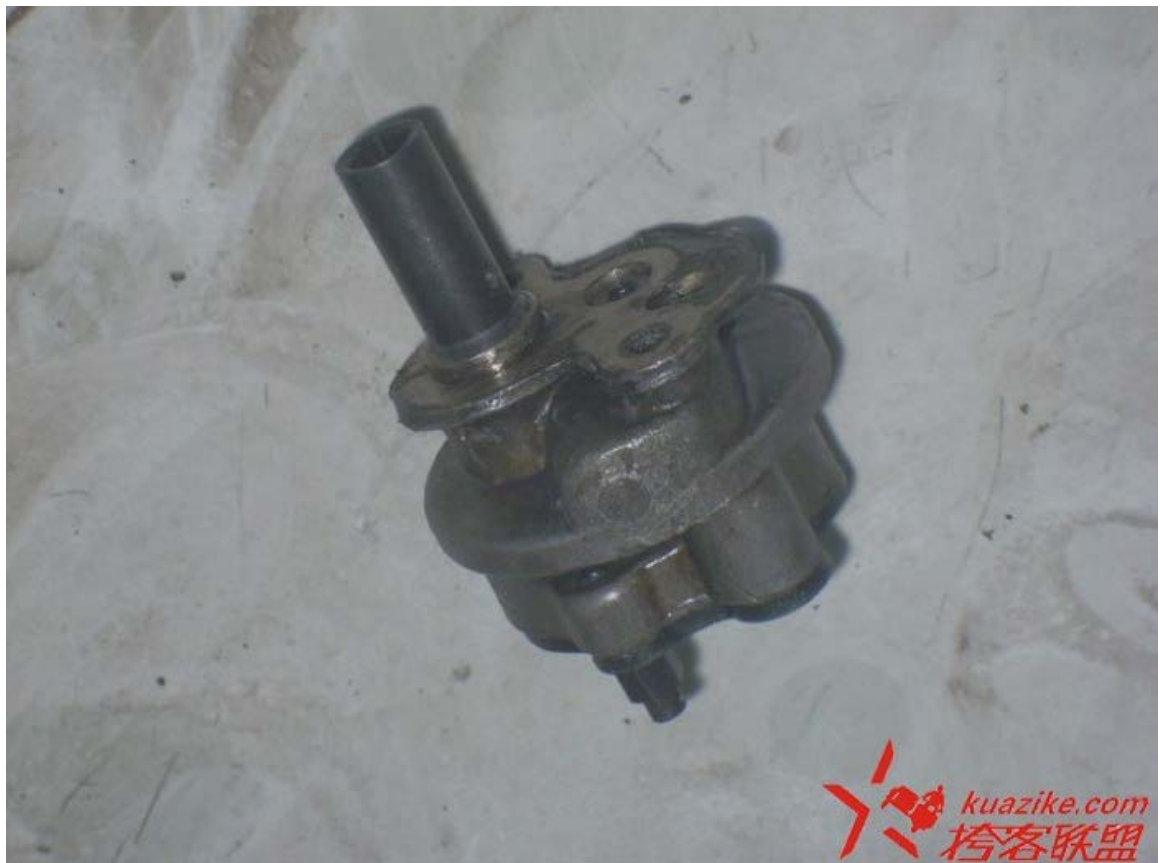
32P的机油泵，这是清洗检查过后的。 The OHV oil pump after cleaning and inspection.
