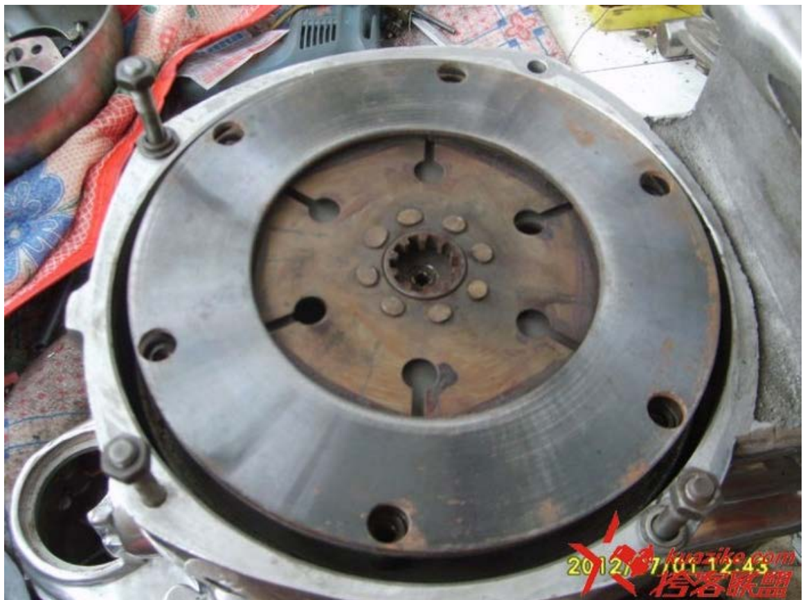
放上中间的离合铁片，要对准上下固定孔。Place the pressure plate lined up with the screw posts.
