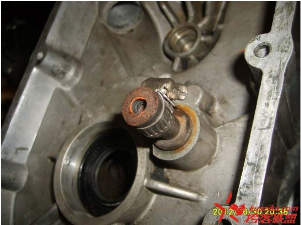
用卡子扎紧油道接头，防止漏油。 A hose clamp was added as added assurance against leakage.
