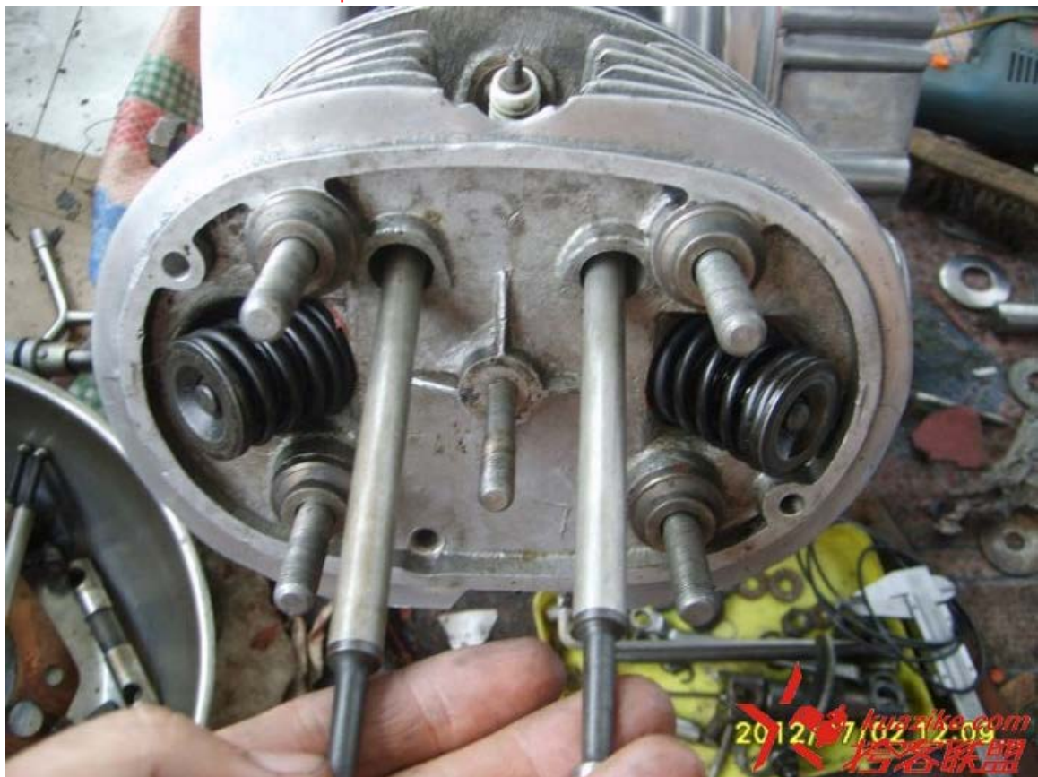
装上汽缸垫，这一张漏拍了！ 😊 注意缸垫上的回油孔必须和缸桶的油孔对准！！ 然后装上汽缸盖，并插入气门顶杆。 Forgot to take a picture! Note that the cylinder base gasket has a hole that must be aligned with the oil return tube on the underside of the cylinder. Next, mount the head, and insert the pushrods.
