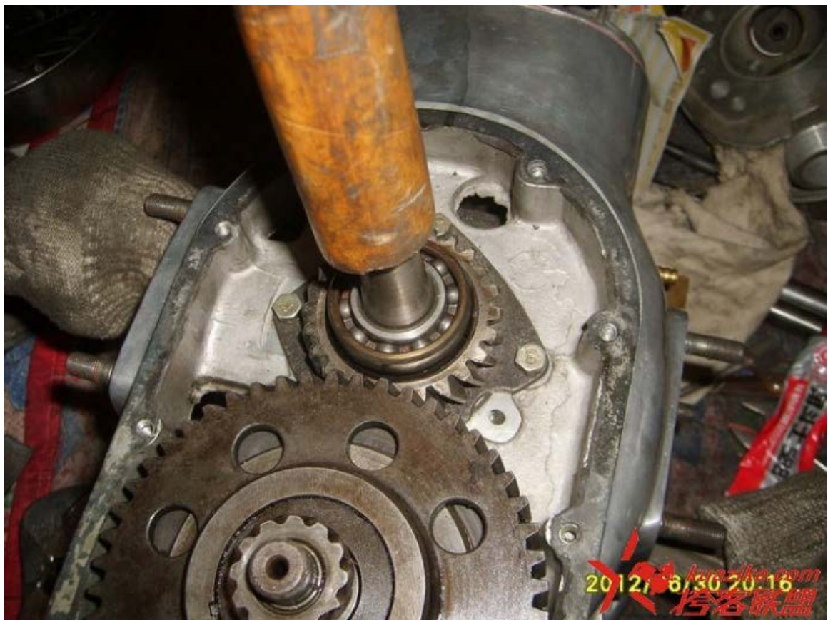
用木棒把发电机轴震到位。Tap the alternator shaft in place.
