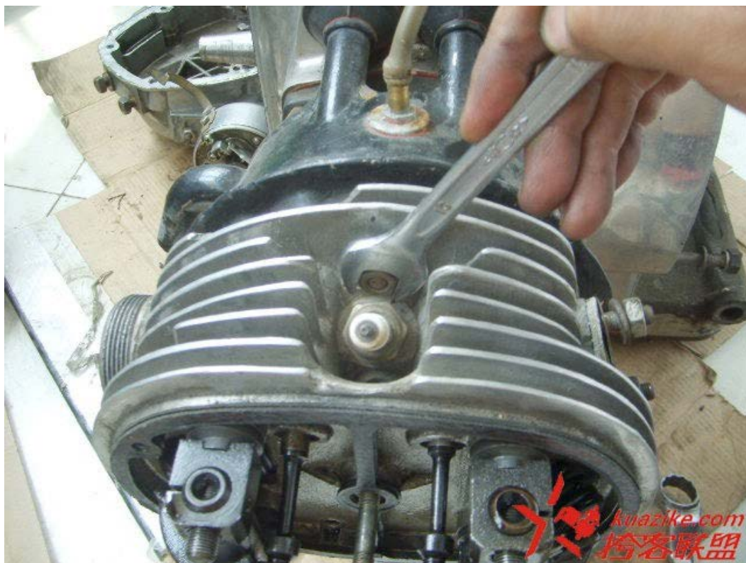
拆下上火花塞旁边的13MM螺母 Use a 13mm wrench to remove the nut behind the spark plug.
