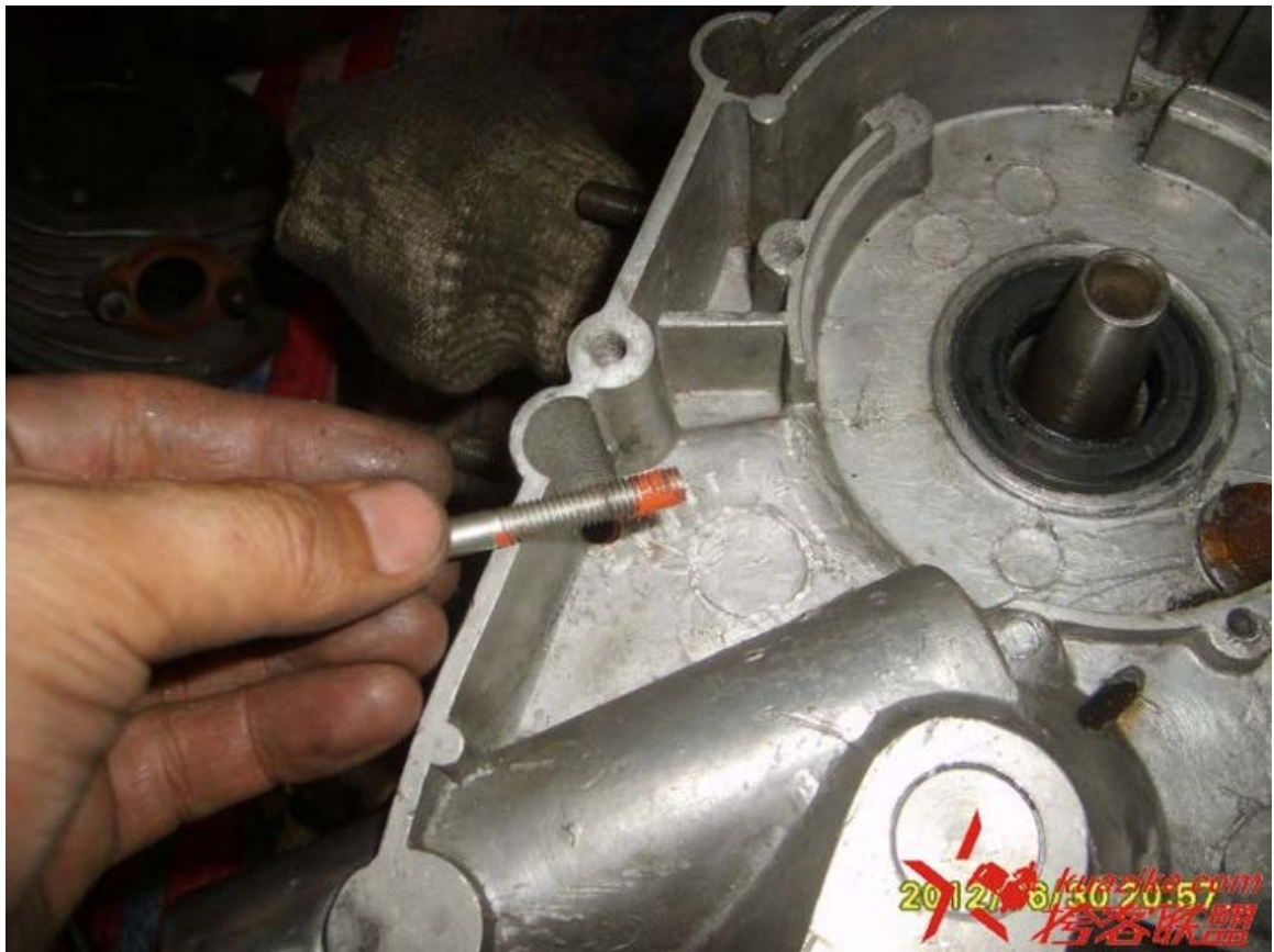
前机盖固定螺丝全部挂胶在上紧 Sealant added to the front cover bolts.
