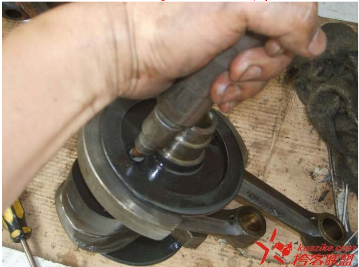
用冲击起子拆下曲轴前后挡油盘。 Use an impact screwdriver to remove the oil slingers.
