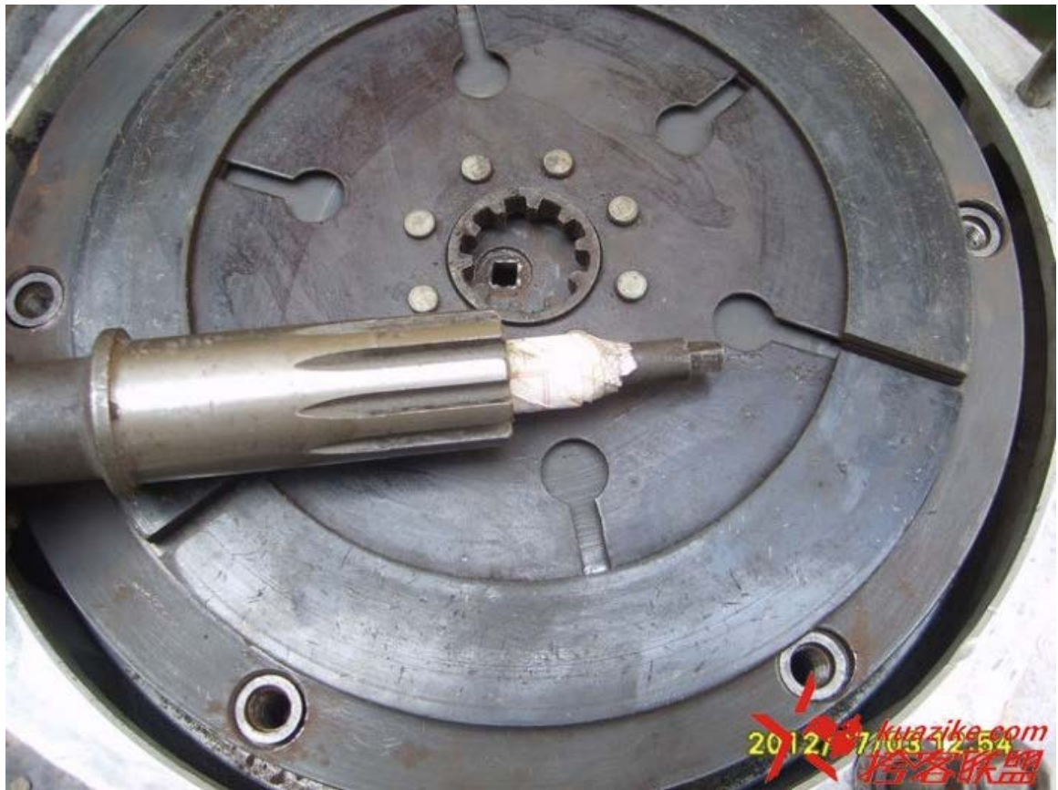
为了准确对准两个离合片与压盘顶杆孔的位置，使用了变速箱一轴和离合顶杆，离合顶杆缠几层硬纸再插入一轴内，可以保证顶杆和一轴同心。The friction and pressure plates must be correctly aligned. Here a clutch push rod wrapped in paper inside a gearbox shaft is used as an alignment tool.
