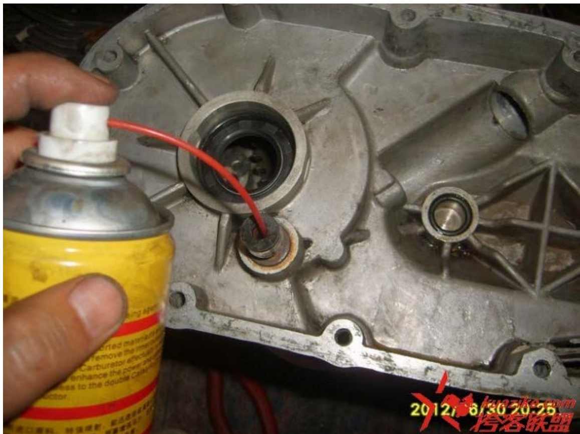
用清洗剂清理前机盖油道。 Clean out the oil channel before assembling the front end.
