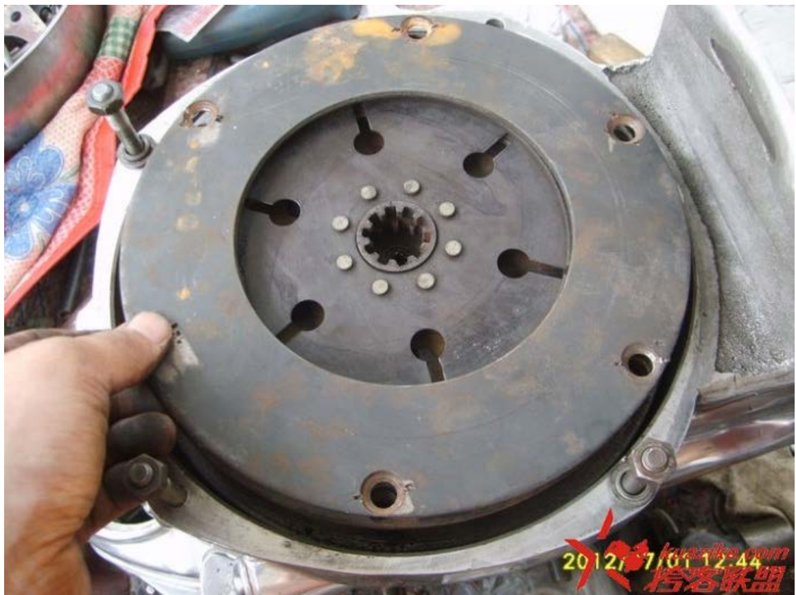
放上 上离合压盘，三层的固定孔都要对齐。The pressure plate is lined up with the bolt holes.
