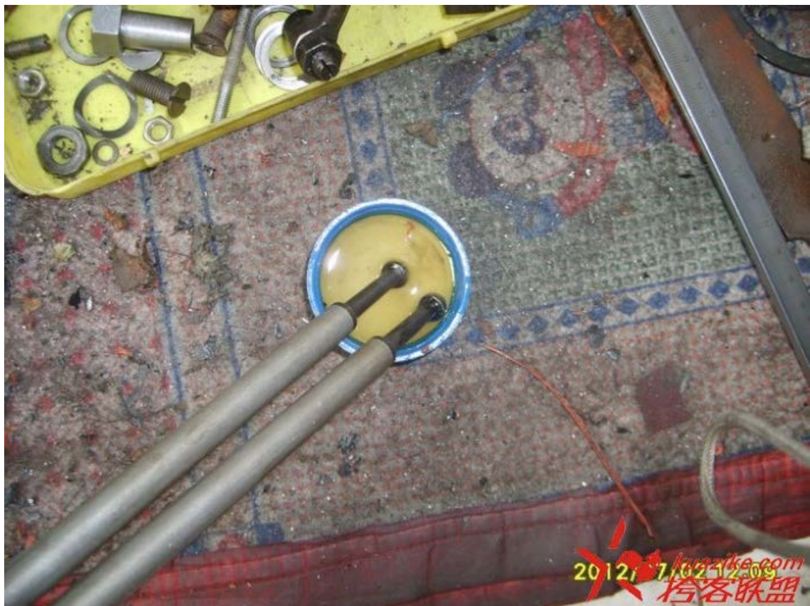
气门顶杆两头沾机油。 Grease the pushrod ends.
