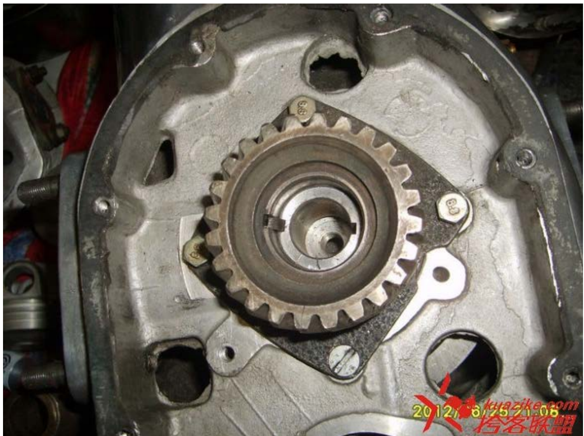
装上正时齿轮 Fitting the timing gear to the crankshaft.
