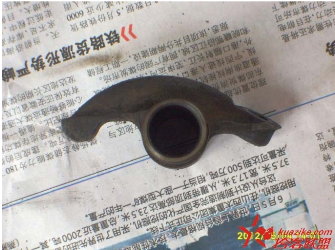
有很多多余的部分可以用作减肥处理。 There is excess metal that can be trimmed off to reduce weight.
