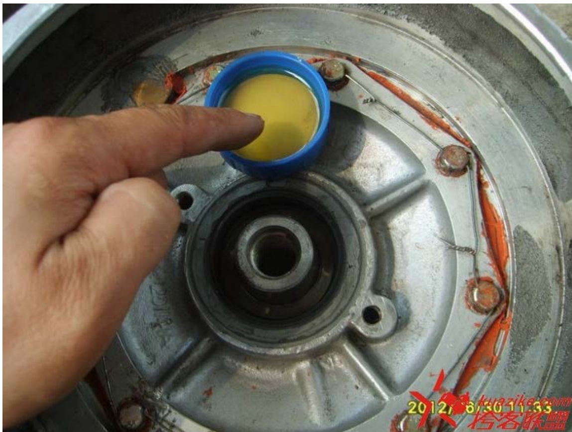
抹点机油给油封润滑 Lubricate the oil seal surface.
