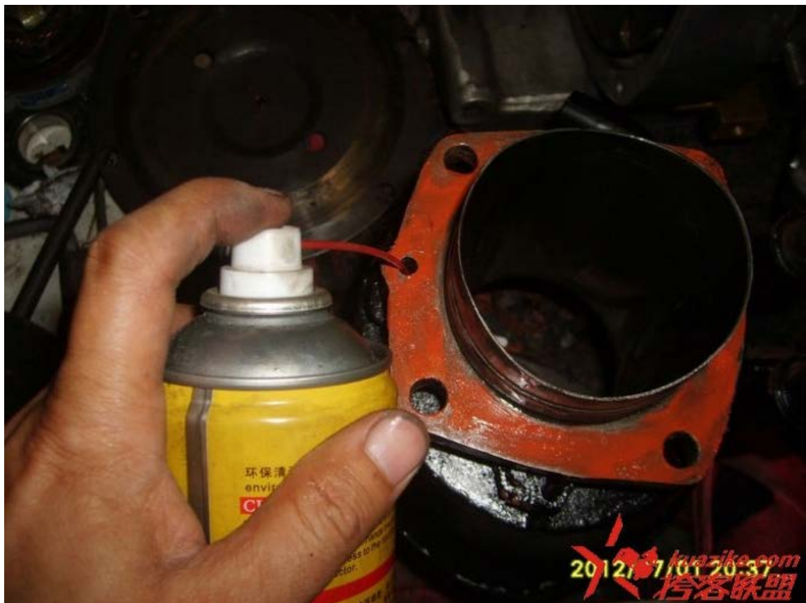
清洗缸桶的回油油道 Cleaning the oil return channel on the underside of the cylinder.
