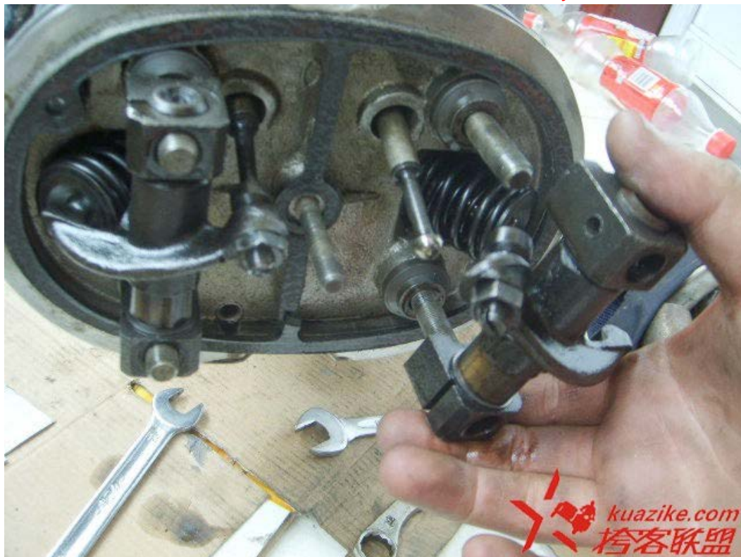
拿下气门摇臂组合，注意按照位置摆放好，方便检查和清洗。 Remove the rocker arm assembly for cleaning, noting the position of the various components.
