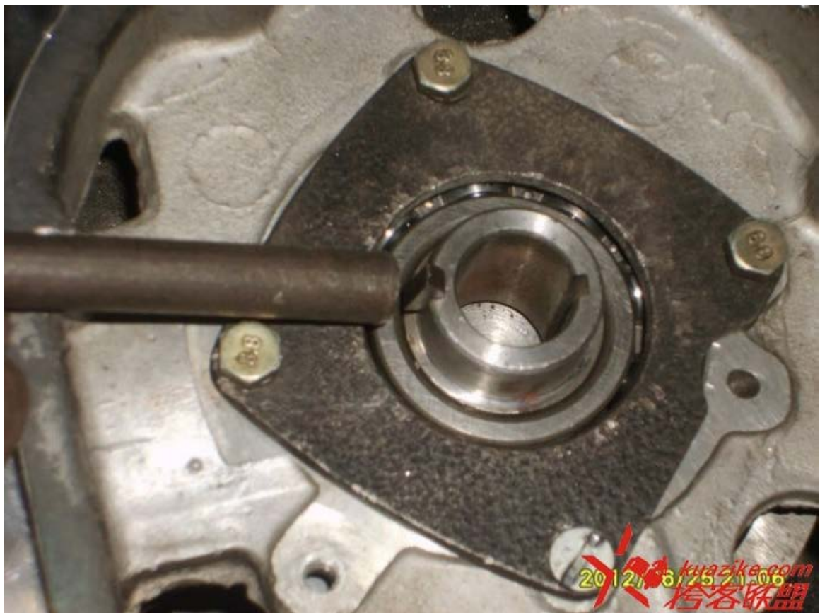
装上曲轴 正时齿轮的定位键。 Place the timing gear's Woodruff key on the shaft.
