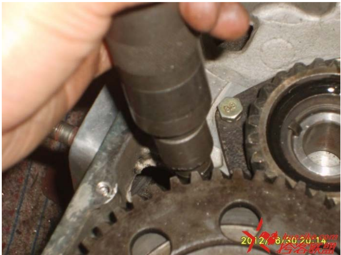
用冲击起子锁紧。 Tighten with an impact screwdriver.
