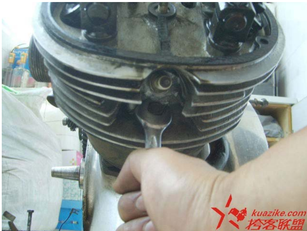
缸盖下部的13MM固定螺母 Use a 13mm wrench to remove the lower cylinder head nut.
