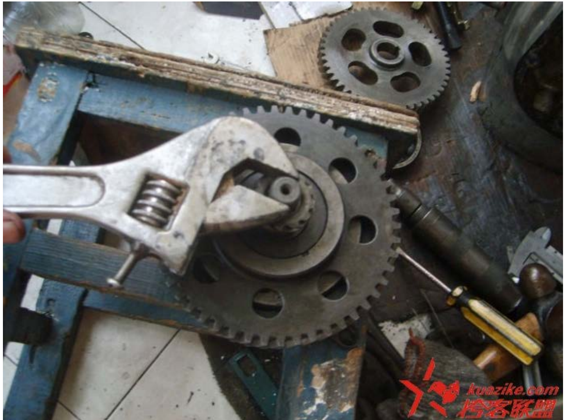
装上分电器传动涡轮。 Fitting the distributor drive gear.
