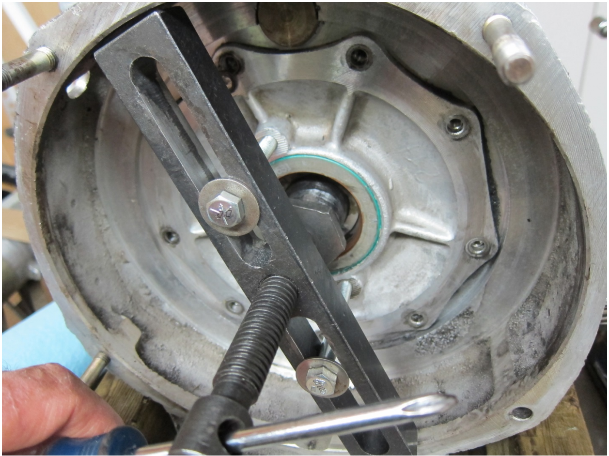
Figure 6 - Pull the bearing plate using the puller from the tool kit
