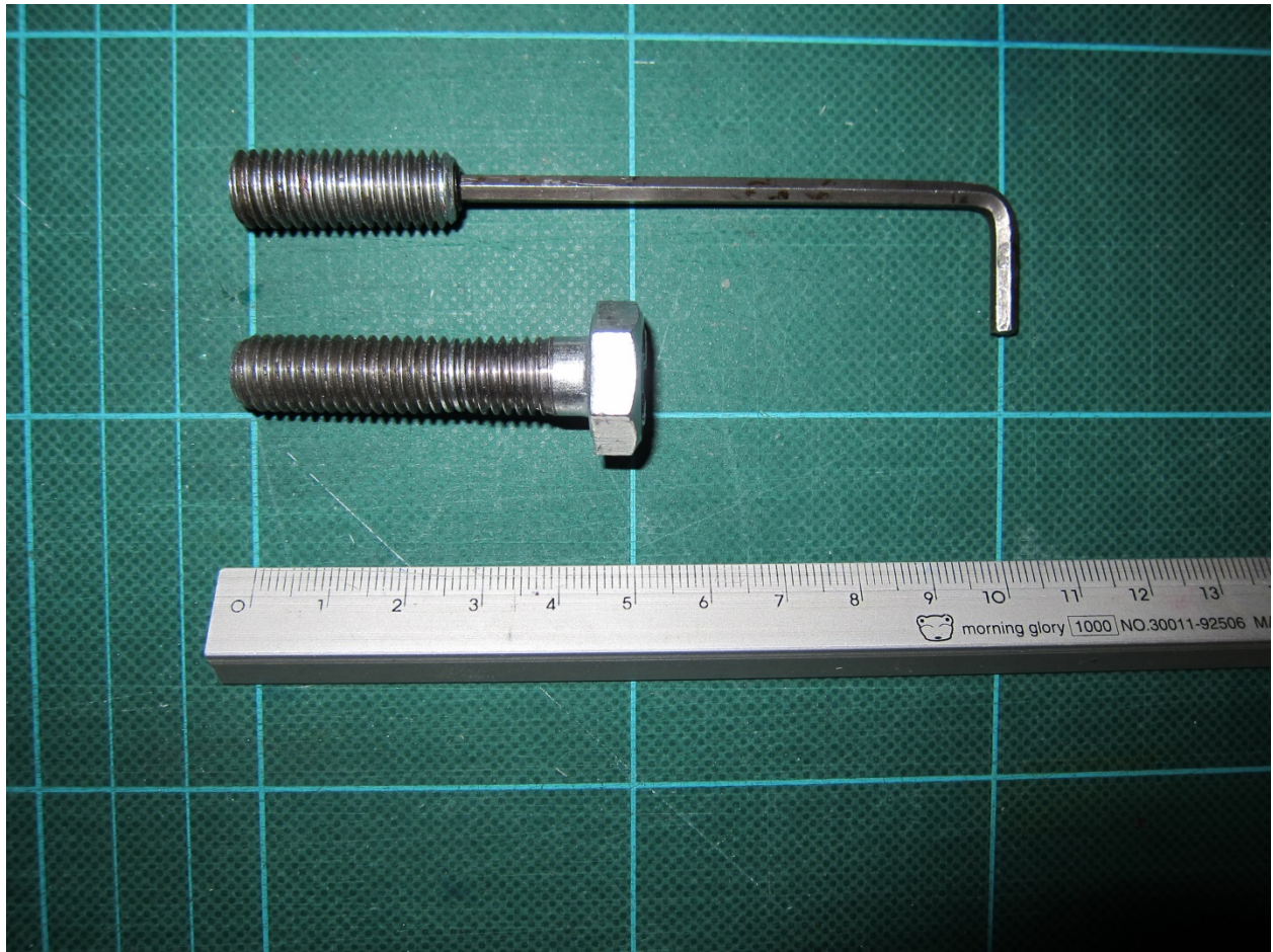
Figure 12 – Bolts used to remove the alternator rotor from its shaft
