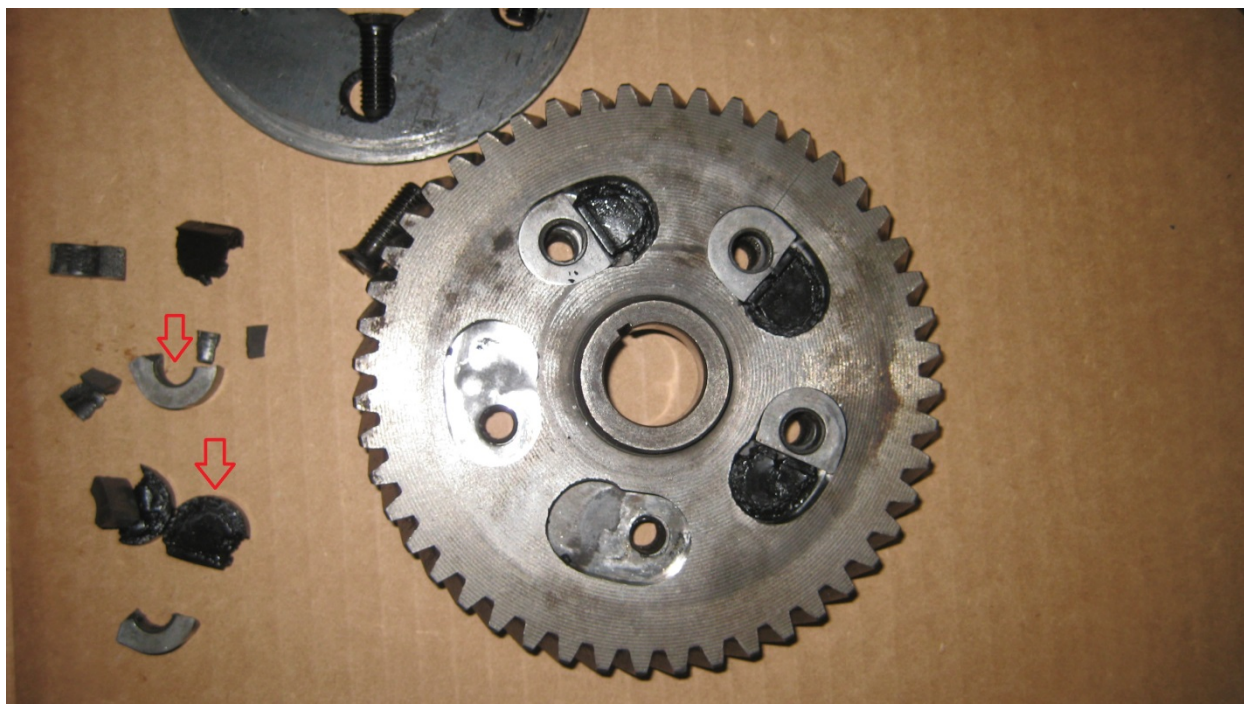
Figure 18 - Starter free-wheel clutch showing broken damper parts
