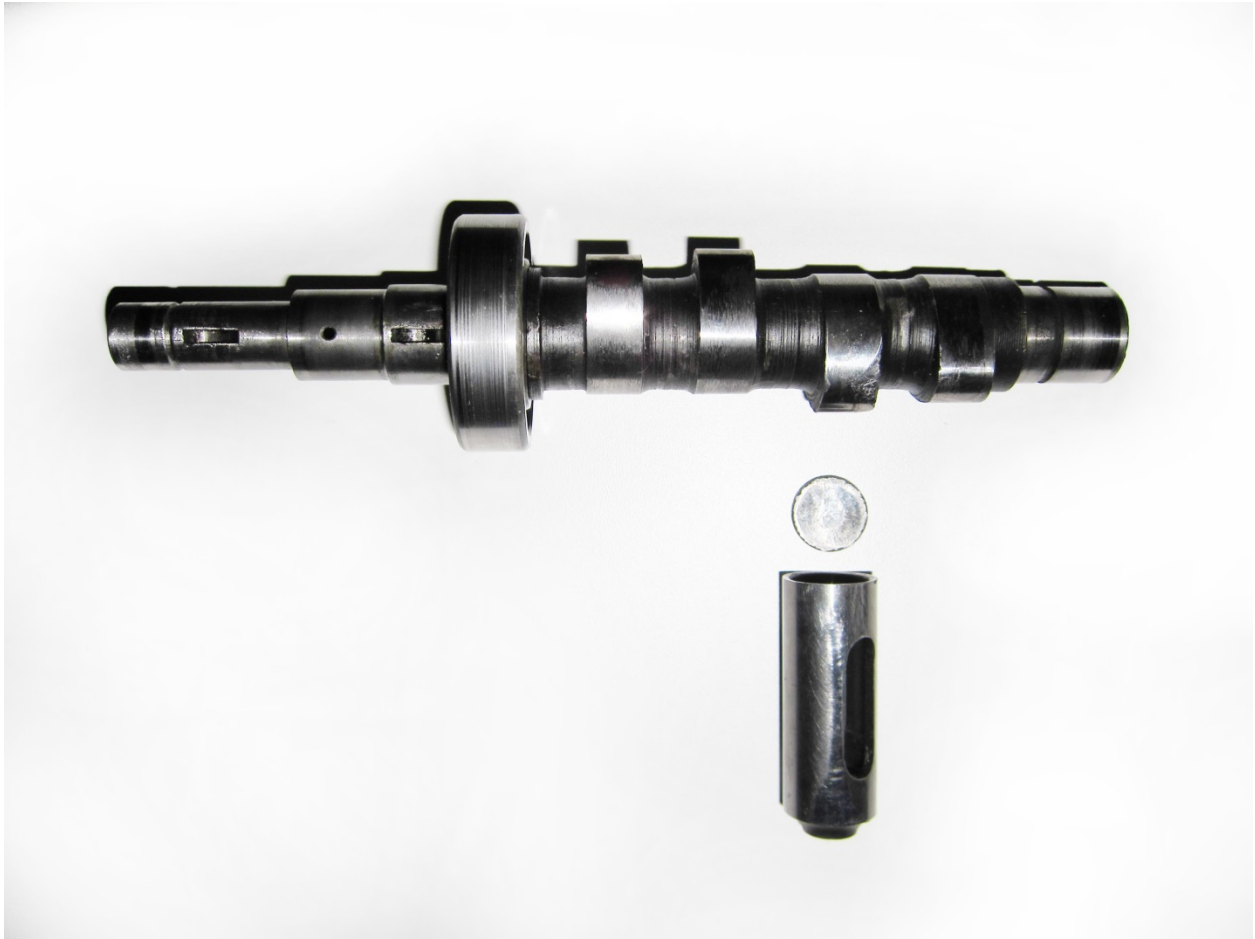
Figure 14 - Broken tappet and damaged cam lobe
