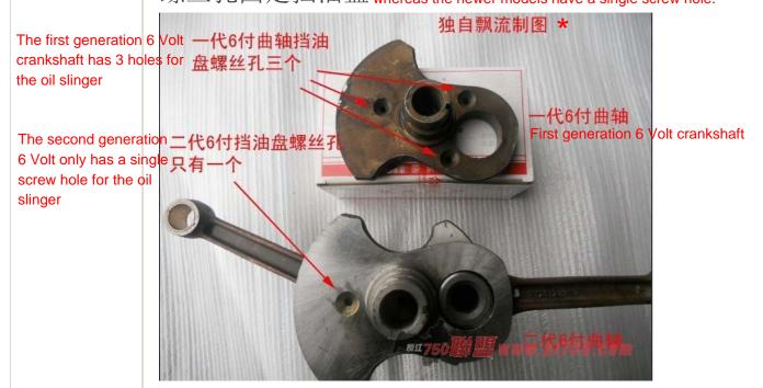
Differences between first and second generation 6 Volt crankshafts 一代和二代6付的曲轴箱体有所不同
