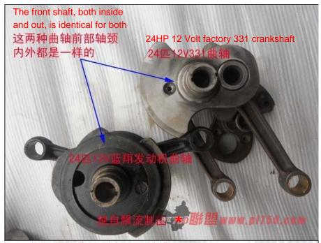
The keyway on the Lanxiang crankshaft is longer and wider than one from factory 331
