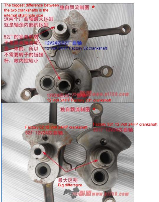
The keyway on the front of the factory 52 crankshaft is slightly wider and a little longer
