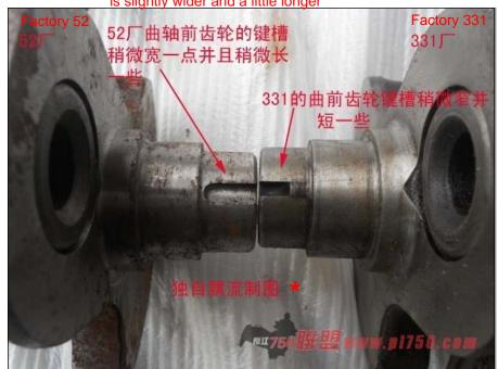
The keyway on the factory 331 crankshaft is shorter and narrower
