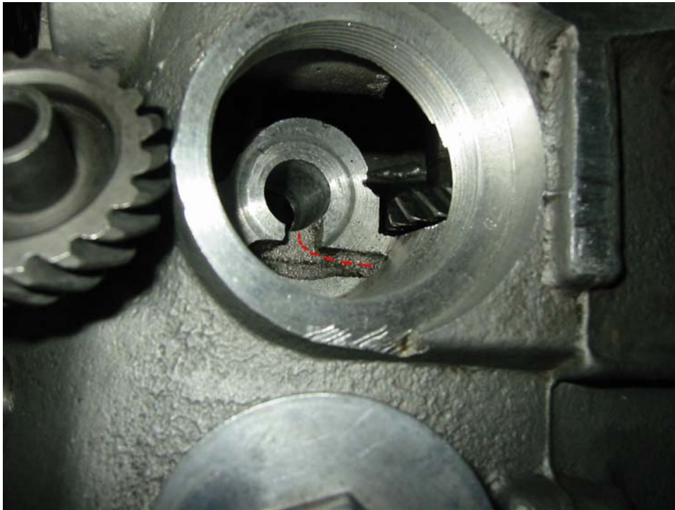
Figure 11 - Pump gears and camshaft bushing lubrication
