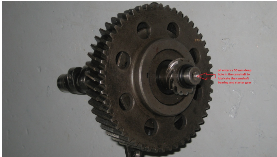
Figure 8 - Starter freewheel clutch lubrication
