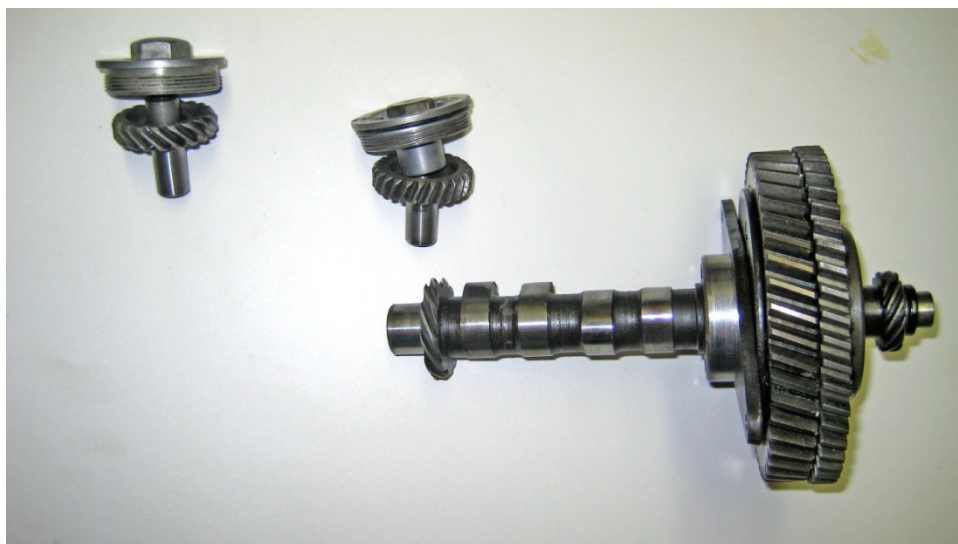
Figure 1 - oil pump gears
