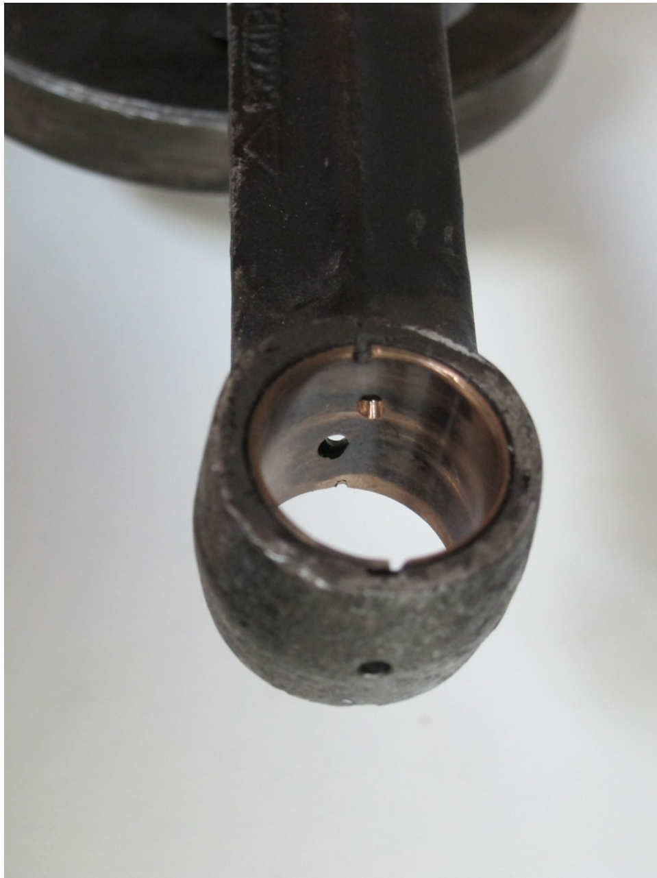
Figure 12 - Wrist pin lubrication
