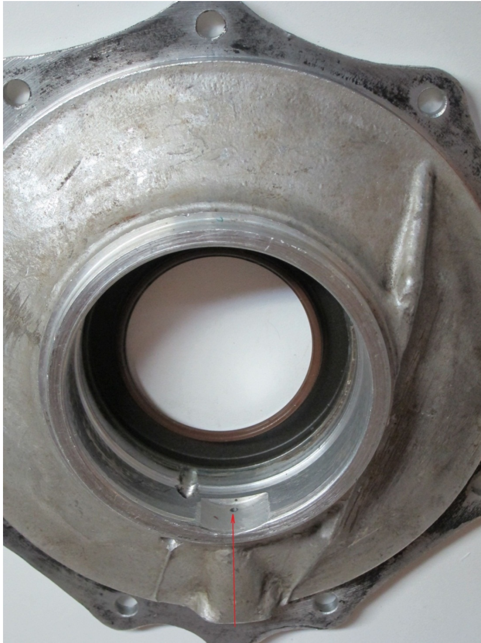
Figure 4 - Rear bearing lubrication
