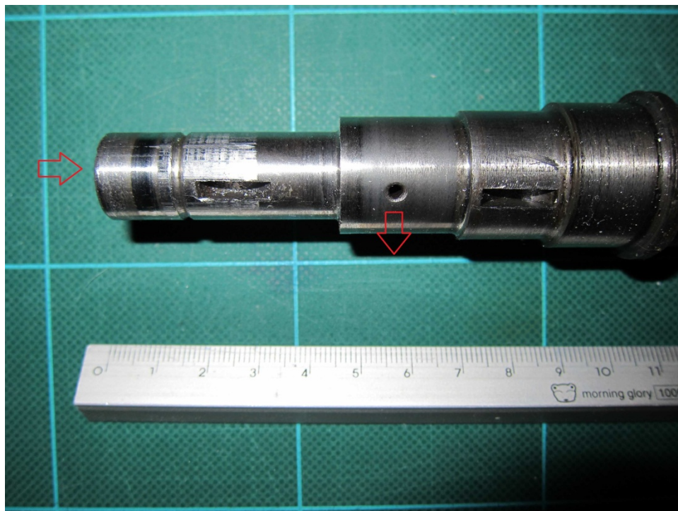
Figure 9 - Detail of camshaft oil conduit
